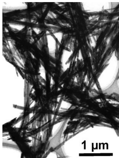
Fig. 4 Representative TEM image of molybdenum oxide fibers which have been heated at 400 °C for several hours in air.
